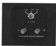
In rooms that are paneled, where hard surfaces abound, or in sparsely furnished rooms, or if very bright sounding source material is normally used, you may find that the "-3" or \*-6" positions of the switches will result in best overall music balance
